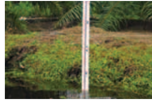
Figure 9: Water level gauge for water level monitoring in collection drain.
