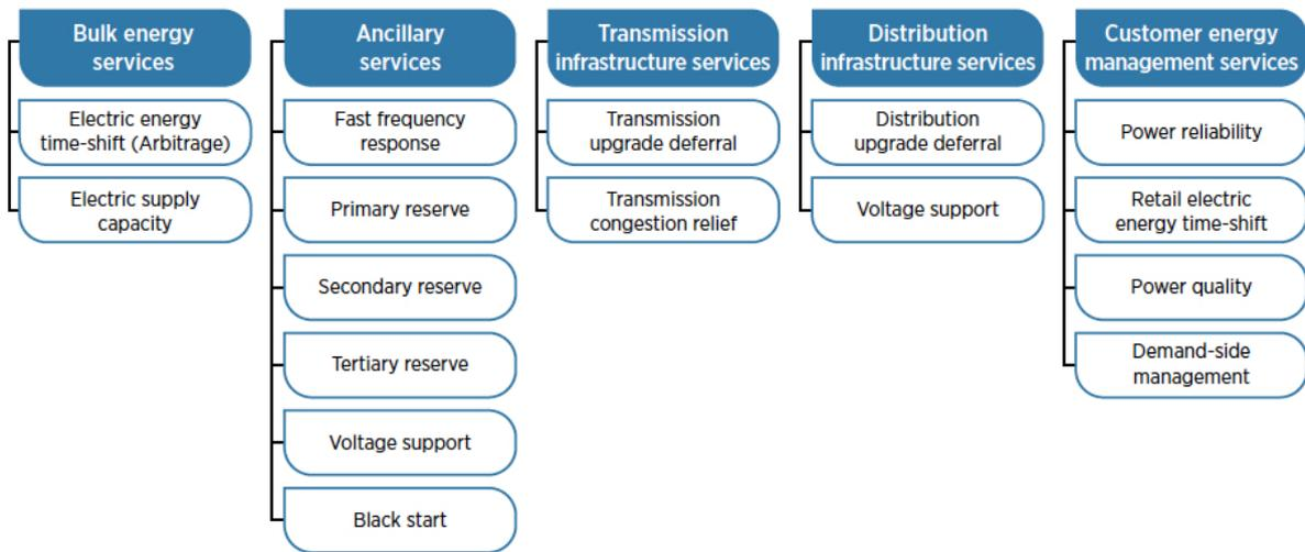
Figure 3: Functions of battery storage
