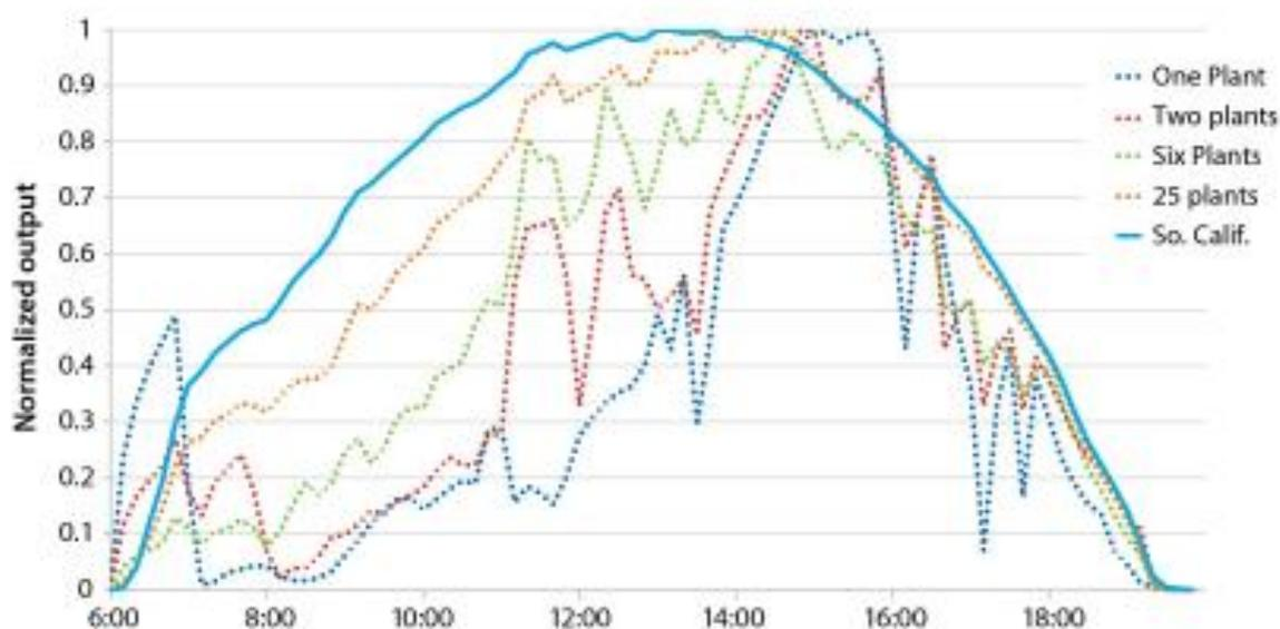
Figure 1: Output profile of different solar PV projects, including in all of Southern California
