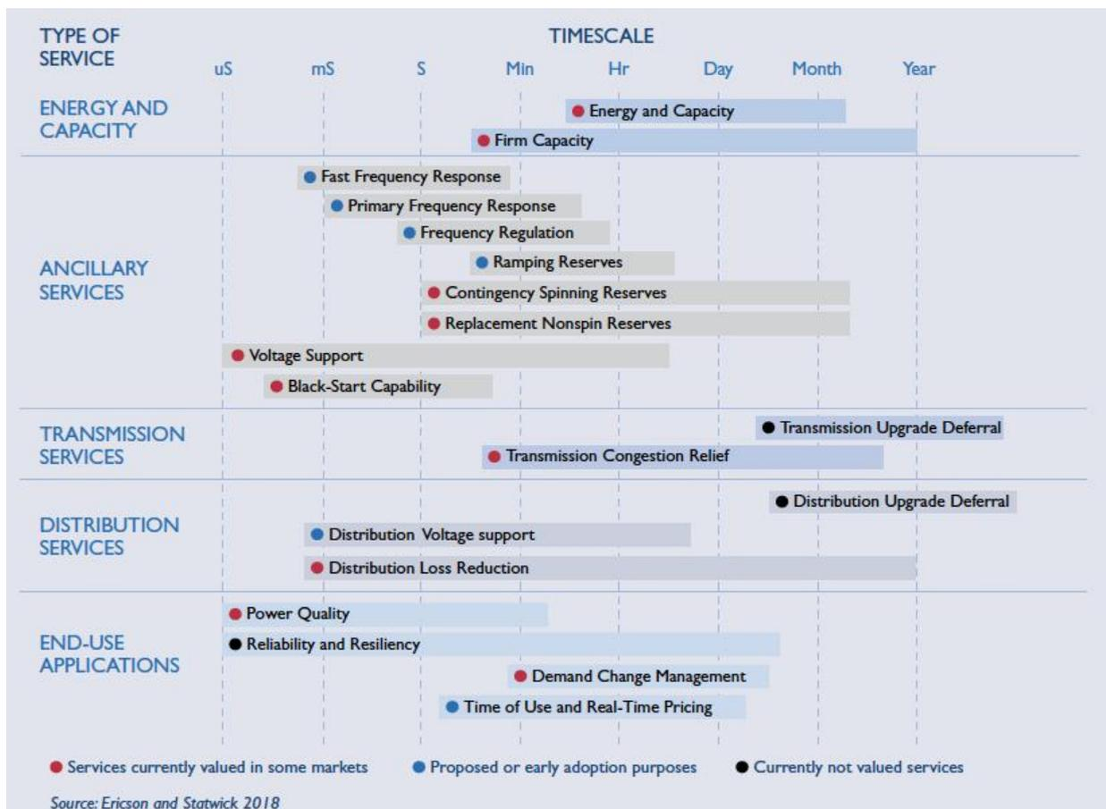
Figure 4: Timescale over which different battery storage services are provided
